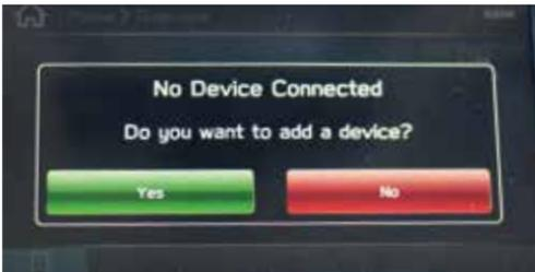
A Bluetooth PIN will appear on the screen. Put your phone into Bluetooth pairing mode. Follow the prompts on your phone screen to pair your phone to the vehicle system using the PIN shown on the screen.
