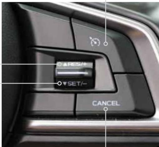
Press the accelerator pedal until your vehicle reaches the desired speed. Push the switch to the “SET” side and release. Ease off the accelerator pedal. Your vehicle will maintain the desired speed.
