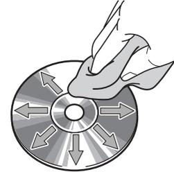
**To clean a disc:** Wipe it with a soft, lint-free cloth that has been dampened with water. Wipe in a straight line from the center to the edge of the disc (not in circles). Dry it with another soft, lint-free cloth. Do not use a conventional record cleaner or anti-static device.
