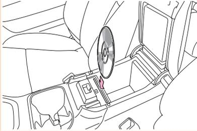
Insert the disc with the label side facing the rear of the vehicle.
