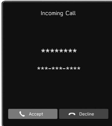
**To refuse to receive the call:** Select **Decline** (Decline) or press the
