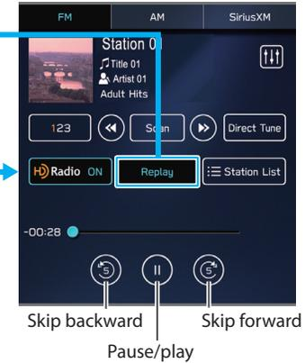
Depending on the radio broadcast, the broadcast can be temporarily saved and played back later. P.161
